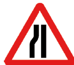
Road narrows on left ahead
