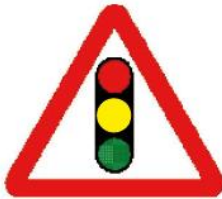
Traffic signals ahead
